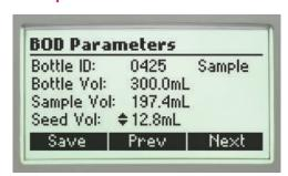
All necessary parameters for BOD testing can be set and displayed at once.
