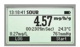
Measured in mg of oxygen consumed per g of volatile suspended solids per hour.
