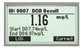
BOD is calculated in mg per liter from the difference between the initial and final dissolved oxygen concentration readings.
