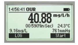
Measured in mg of oxygen consumed per L per hour.
